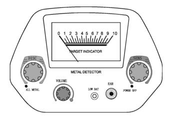
DISC (Recognition Search Mode). Turn the knob clockwise from the ALL METAL point to the right to enter DISC mode. Rotate the knob clockwise slowly to track out false signals from (interference, debris, etc.).
