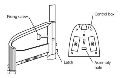
4. Tighten the fixing screw on the handle.
